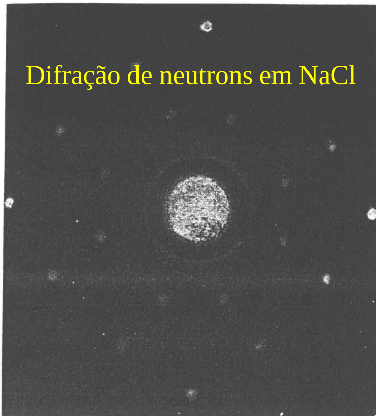
FIGURE 4.4 Diffraction of neutrons by a sodium chloride crystal. [Source: Eisberg & Resnick, Quantum Physics , John Wiley & Sons, 1974.]
