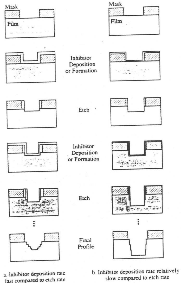
**Figure 10-14** Illustration of the effect of the inhibitor deposition rate-to-etch rate ratio on the resulting sidewall slope. The different relative rates of inhibitor deposition and etch rate lead to different slopes of sidewall [10.4].
