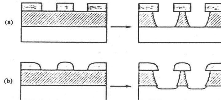
**Figure 10-2** Actual etch profiles that can occur. (a) Lateral etching under mask. (b) Rounded photoresist which is further eroded during etching, leading to even more lateral etching. (b) also illustrates etch selectivity.
