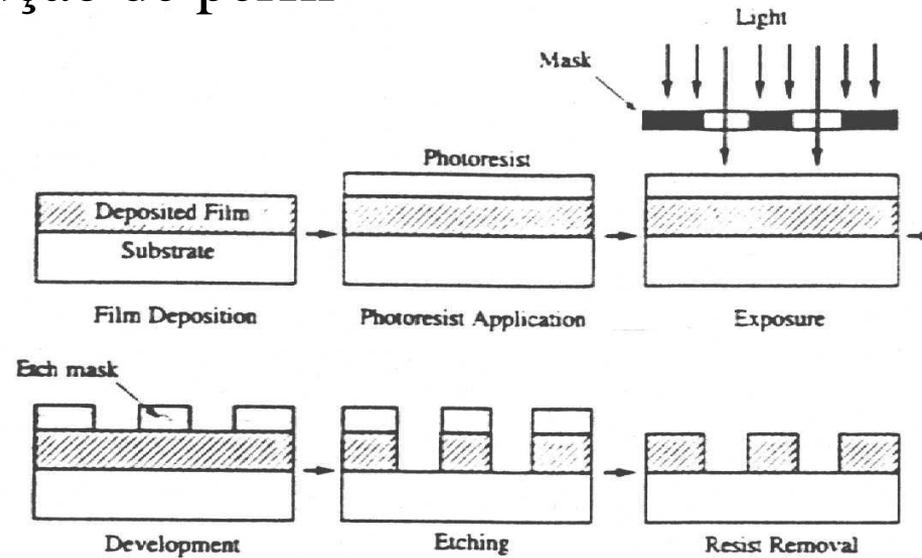
**Figure 10-1** General process used in integrated circuit fabrication to define patterned films.
