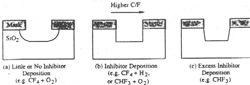
**Figure 10-24** Effect of inhibitor deposition on resulting etch profile. The profiles shown assume no mask erosion, which may occur for different etch chemistries. The actual profiles obtained will also depend on the specific etch system and plasma conditions.
