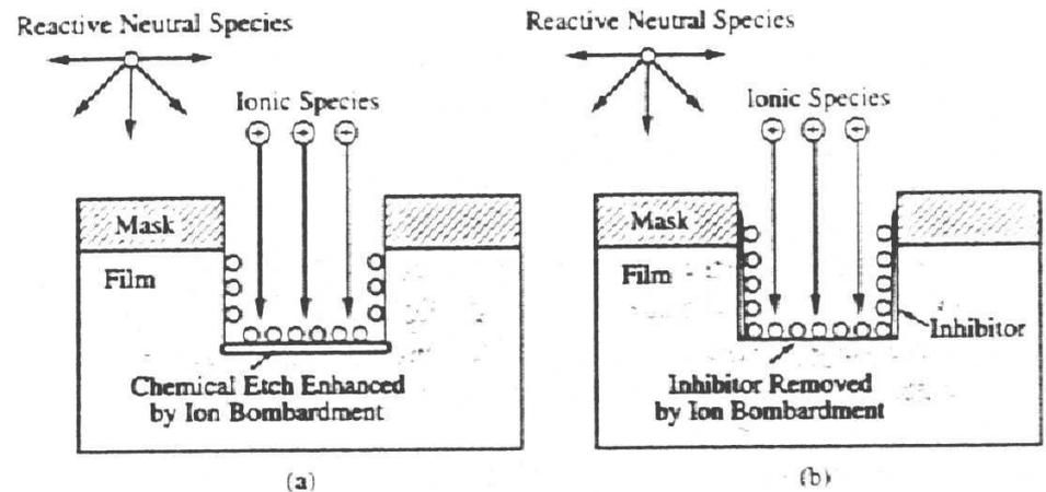
**Figure 10-13** Illustration of ion-enhanced etching. In (a) the chemical etch reaction is enhanced by ion bombardment. In (b) an inhibitor is formed which is removed by ion bombardment, allowing chemical etching to proceed. In both cases, anisotropic etching results.
