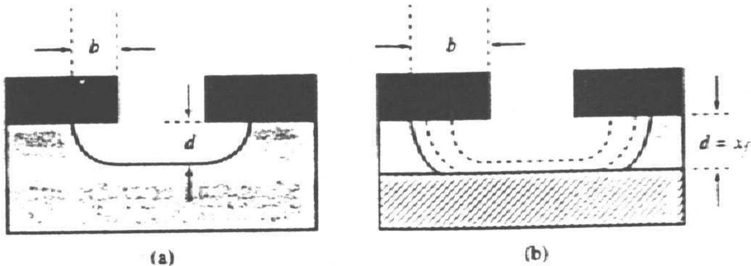
**Figure 10-4** Illustration of etch bias and overetch. In (a) the etch bias,  $b$ , is shown for a given etch depth,  $d$ . In (b), overetching is illustrated where etching is continued even after the etch depth,  $d$ , equals the film thickness,  $x_f$ , with the result that the etch bias increases.
