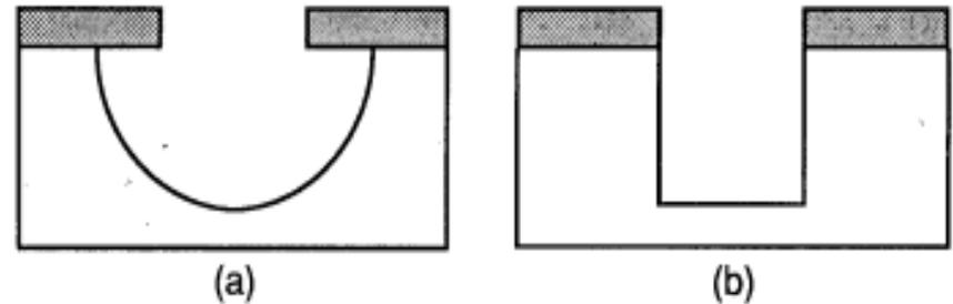
Schematic illustration of (a) isotropic and (b) vertical etching.
