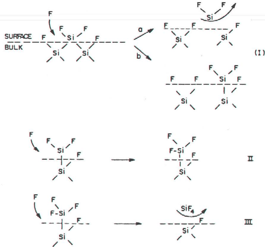
Fig. 7 Proposed mechanism for F-atom reaction with a silicon film leading to the products SiF<sub>2</sub> and SiF<sub>4</sub><sup>13</sup>. Reprinted with permission of the American Physical Society.
