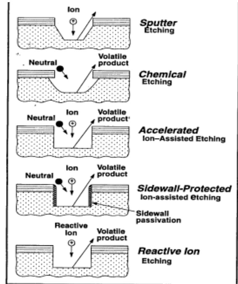
Illustration of plasma etching integrating chemical and physical etching.
